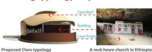
The separate class room typology is inspired from the ancient rock cut and rock hewn churches in Ethiopia and ancient temples on ancient Egypt. The class room is sandwiched between the overhanging roof and the short space defining wall. This approach creates the hidden rock cut African architecture. Inspires the students to look back through history and search for inspirational knowledge
